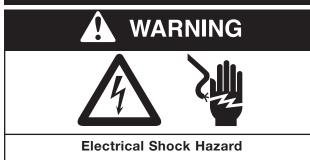
Disconnect electrical power at the circuit breaker or fuse box before installing this product.
