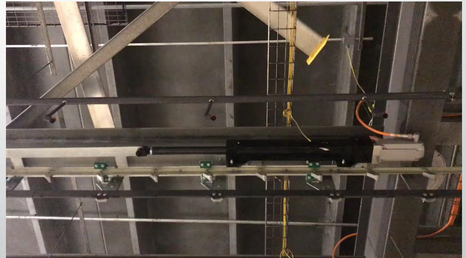
Servo Driven Electric Walking Beam
