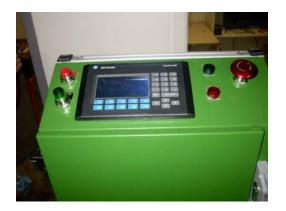
stop button (the operator cannot stop the test until at least ten minutes have passed). When the operator stops the test, the pressure reading at the end of test, the time of test, and pressure loss during the test are displayed on the operator interface. A red (fail) or a green (pass) indicator will also light and the unit being tested will depressurize. The operator can then either repair the unit or send it to be installed on the machine.
