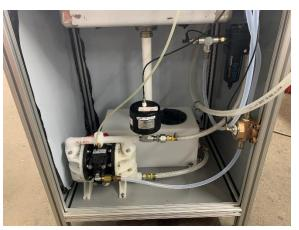
3. CMD added a dampener to the diaphragm pump to reduce the chugging that naturally occurs with this style of pump for a smooth consistent water flow.
